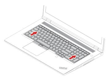
3. Pivot the keyboard slightly upward  $\blacksquare$  and then turn the keyboard over  $\blacksquare$ .
