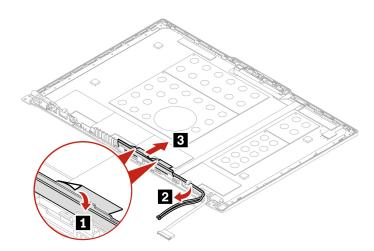
Attention: When you route the cables, ensure that they are not subject to any tension. Tension could cause the cables to be damaged by the cable guides, or a wire to be broken.
