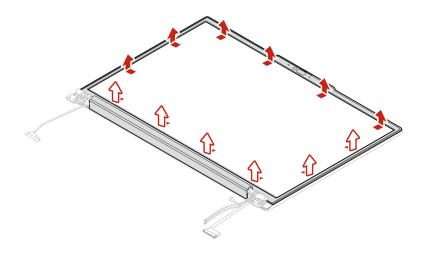
Step 2. Install the LCD bezel in reverse order.
