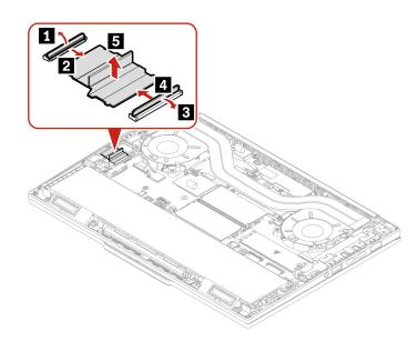
Step 2. Install the I/O board cable in reverse order.
