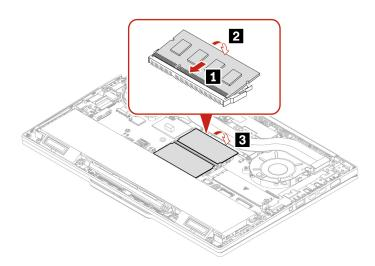
Note: Memory module replacement might cause memory retraining during POST. When memory retraining occurs, the screen might be blank. You might see the LED indicators on Esc, F1, and F4 blinking sequentially to indicate the progress. Do not press the power button to interrupt the process. Wait a few minutes until the logo screen is displayed.
