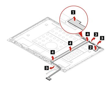
Step 2. Install the camera-and-lid cable in reverse order.
