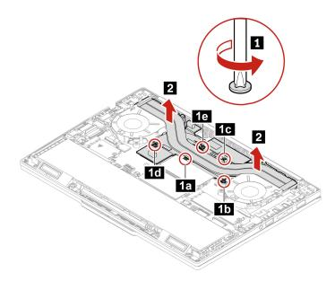
Step 2. Install the thermal assembly in reverse order.
