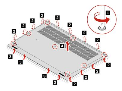
**Note:** Prepare a pry tool to release the hooks.
