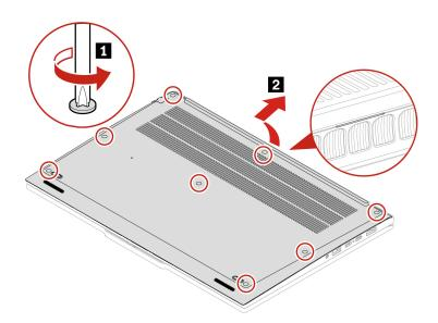
Note: If the base cover assembly cannot be opened by hand, use a pry tool to assist.
