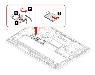
Note: A mylar film might cover the wireless WAN module. To access the wireless WAN module, peel off the film first.
