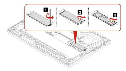
Step 2. Install the M.2 solid-state drive and its bracket in reverse order.
