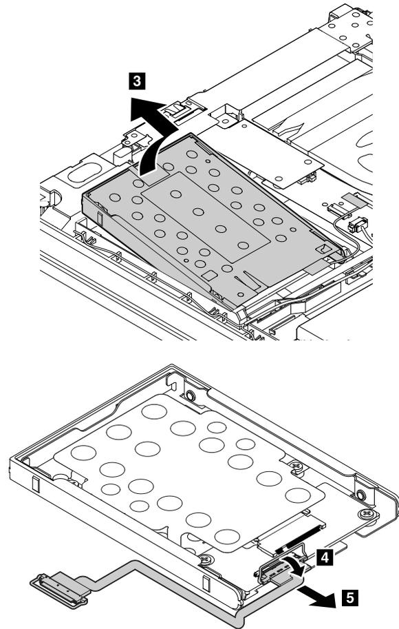
**When installing:** Ensure that the storage drive is firmly attached.
