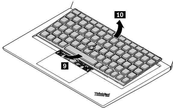
8. Put the keyboard on the palm rest as shown. Open the plastic shield and detach the connectors. Then remove the keyboard.
