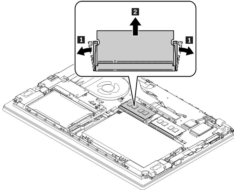
**When installing:** Insert the notched end of the memory module into the memory slot at an angle of about 20 degrees. Press the memory module in firmly, and pivot it downward until it snaps into place. Ensure that the memory module is firmly installed and does not move easily.
