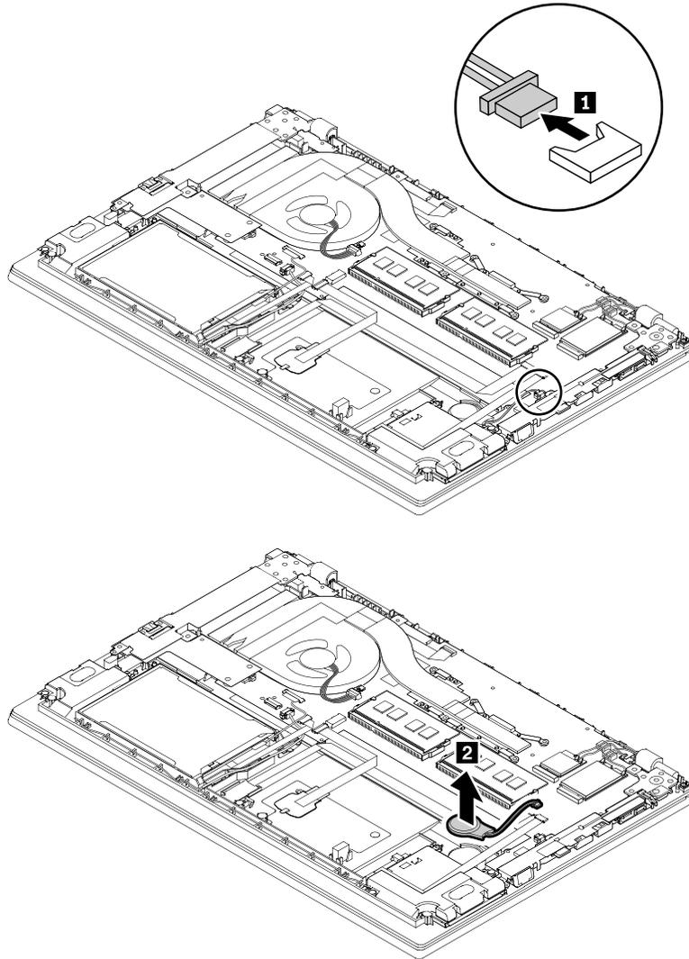
**When installing:** Ensure that the connector is firmly attached.
