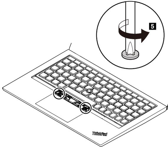
4. Insert the tabs **c** and **d** into the two dents near the two screw heads **6**.
