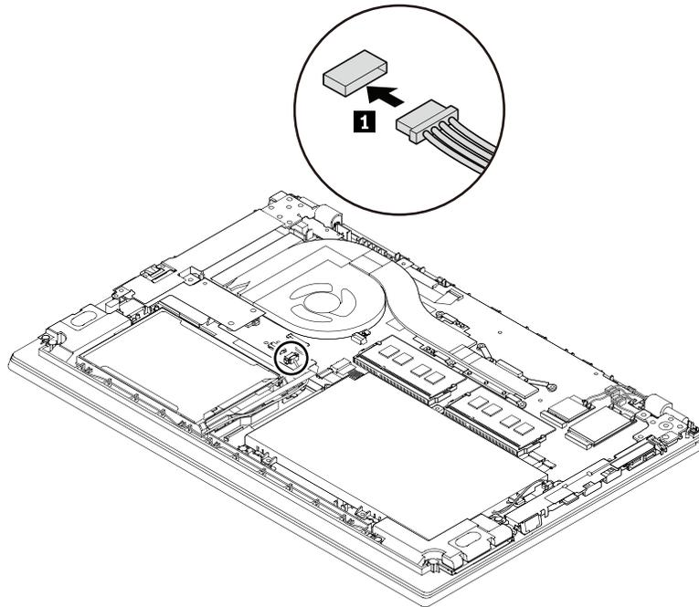
**When installing:** Ensure that the connector is firmly attached.
