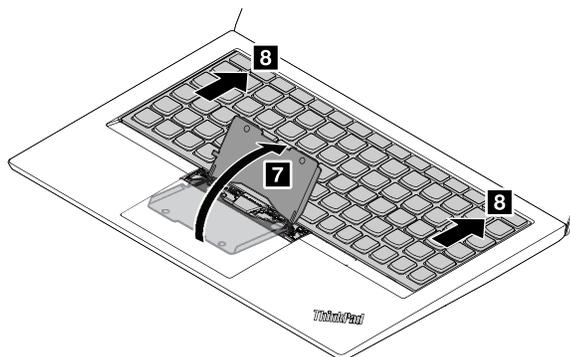
6. Pivot the tool in the direction as show to release the keyboard **7**. Push the keyboard in the direction as shown by arrows **8** to release the latches from the keyboard bezel.
