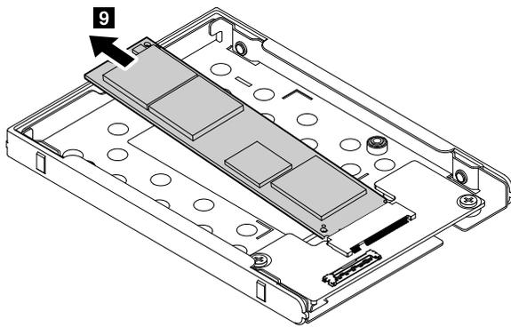
**Removal steps of the M.2 solid-state drive in the WWAN card slot**
