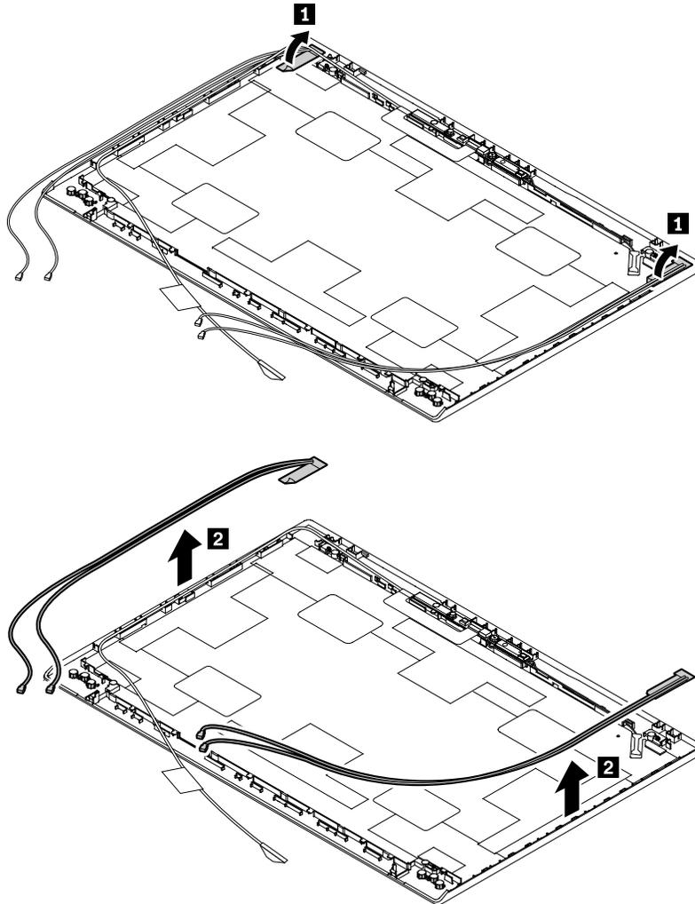
**Attention:** When you route the cables, ensure that they are not subject to any tension. Tension could cause the cables to be damaged by the cable guides, or a wire to be broken.
