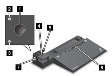
**1 Power button**: Press the power button to turn on or turn off the computer.
