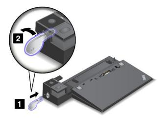
Align the top-left corner of the computer with the position mark of the docking station. Attach your computer to the docking station vertically until you hear a click 1. Then turn the system lock key to the locked position 2.
