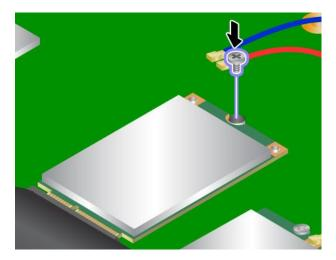
10. Connect the antenna cables to the new card as shown. Then release the hand holding the film.
