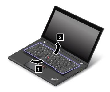
7. Put the keyboard on the palm rest and detach the connectors. Then remove the keyboard.
