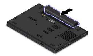
7. Turn the computer over again. Connect the ac power adapter and all cables.
