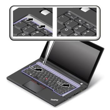
3. Ensure that the screw heads are exposed completely. Otherwise, reveal the screw heads by sliding the keyboard frame forward with the flat-head screwdriver.
