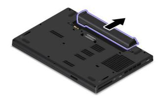
6. Insert a new battery until it clicks into place. Ensure that the battery latches are in the locked positions.
