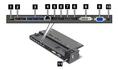
Always On USB connector: Used to connect devices that are compatible with USB 2.0 or charge some mobile digital devices and smartphones when your computer is in sleep or hibernation mode.
