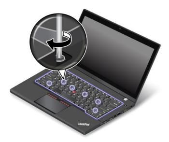
5. Slide the keyboard frame backward by 2.5 mm (0.1 inch) with the flat-head screwdriver to hide the latches of the keyboard frame under the keyboard bezel.
