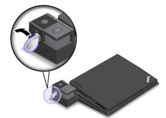
3. Press the eject button until the computer moves up. Then, grasp both sides of the computer to remove it.
