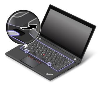
4. Tighten the screws with the cross-head screwdriver to secure the keyboard in place.
