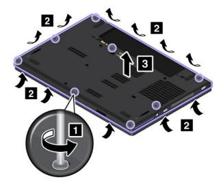
5. Reinstall the computer cover 1. Then tighten the screws 2.
