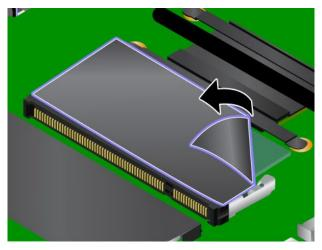
5. Open the latches on both sides of the memory slot at the same time **1**. Then remove the memory module **2**.
