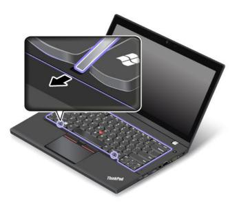
6. Insert the flat-head screwdriver into the sides of the keyboard as shown to push the keyboard frame backward. Ensure that there is no gap between the keyboard frame and keyboard bezel.
