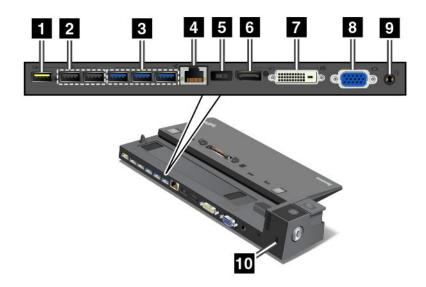
Always On USB connector: Used to connect devices that are compatible with USB 2.0 or charge some mobile digital devices and smartphones when your computer is in sleep or hibernation mode.
