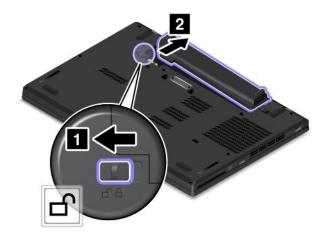
4. Slide the other battery latch 1 to the unlocked position, and detach the battery 2 from the base cover on the right.
