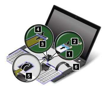
2. Insert the keyboard into the keyboard bezel as shown. Ensure that the front edge of the keyboard (the edge that is close to the display) is under the frame of the keyboard bezel.
