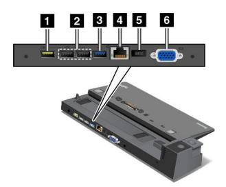
**1** Always On USB connector: Used to connect devices that are compatible with USB 2.0 or charge some mobile digital devices and smartphones when your computer is in sleep or hibernation mode.
