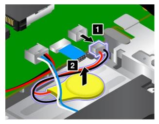
5. Install the new coin-cell battery 1. Then attach the connector 2.
