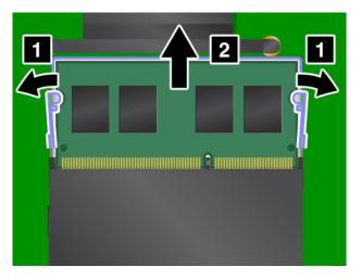
6. Place the notched end of the new memory module toward the contact edge side of the memory slot. Insert the memory module 1 into the slot at an angle of about 20 degrees. Pivot the memory module downward until it snaps into place 2. Ensure that the memory module is firmly installed in the slot and cannot be moved easily. Then release the hand holding the film.
