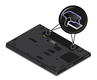
4. Loosen the screws 1. Then remove the cover 2 3.
