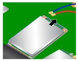
8. Insert the contact edge of the new card to the corresponding socket **1**. Pivot the new card downward **2**.
