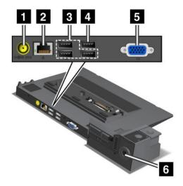
1 Power jack: Connect the ac power adapter.
