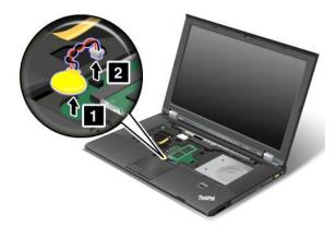
6. Install the new backup battery and attach the connector.
