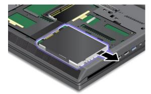
6. Remove the hard disk drive or solid-state drive by lifting its right side.
