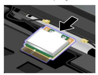
9. Pivot the card until you can snap it into place by pressing the upper side of the connectors, and secure the card with the screw.
