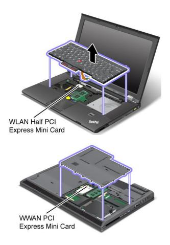
If no integrated wireless PCI Express Mini Card has been preinstalled in your computer, you can install one. To do this, follow the procedure in "Replacing the PCI Express Mini Card for wireless LAN/WiMAX connection" on page 86 or "Replacing or installing the PCI Express Mini Card for wireless WAN connection" on page 88.
