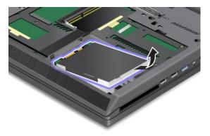
7. Insert the hard disk drive or solid-state drive into the slot.
