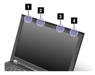
Wireless LAN and WiMAX combo antenna (Main)
