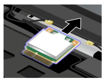
8. Align the contact edge of the new card with the corresponding socket contact of the computer.
