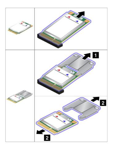
8. Align the contact edge of the new PCI Express Mini Card with the corresponding socket.
