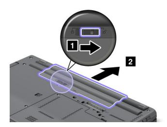
4. Insert a fully charged battery until it clicks into place 1 as shown, and then slide the battery latch to the locked position 2.
