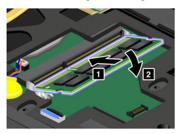
Note: Insert the memory module into the socket at an angle of about 20 degrees.
