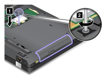
9. Reinstall the cover and tighten the screw.
