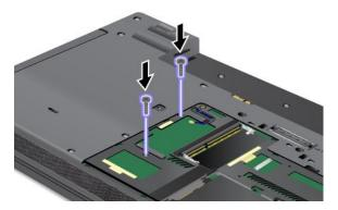
5. Reinstall the cover back into place and tighten the screws.
