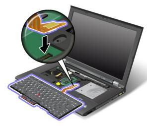
2. Insert the new keyboard. Ensure that the rear edge of the keyboard is under the frame.
