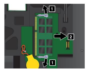
6. Find the notch on the contact edge side of the new memory module you are installing.
