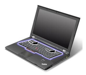
3. Slide the keyboard in the direction shown by the arrows.
