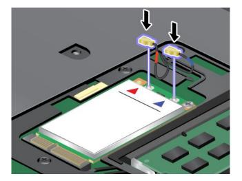
Note: Depending on the model, the marking for the connectors on your card might look different from the one shown in the illustration above. Be sure to attach the red cable to the MAIN or M connector, and the blue cable to the AUX or A connector.
