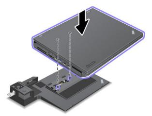
4. Insert your computer into the port replicator or docking station along the surface, until you hear a click. The computer is attached to the port replicator or docking station.
