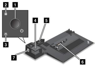
1 Power button: Press this button to turn the computer on or off.
