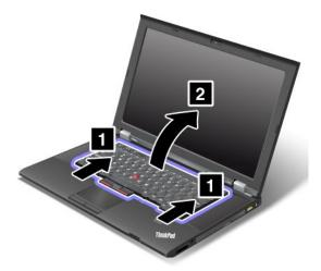
8. Carefully lift the keyboard until you can see how it is connected. Hold the keyboard above the computer, and then detach the connector.
