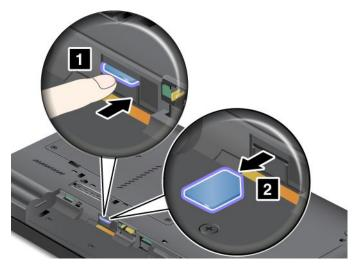
5. Hold the new card with the metal contact facing upward and going into the slot first. Then, insert the card firmly into the slot until you hear a click.
