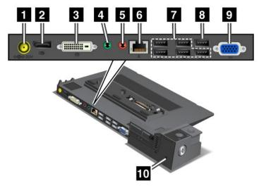
1 Power jack: Connect the ac power adapter.
