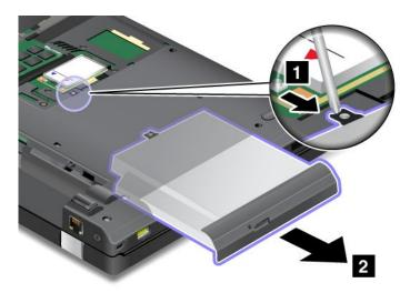
7. Insert the optical drive into the optical drive bay, and then press it firmly into the connector.
