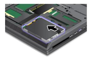
9. Reinstall the cover of the slot, and tighten the screws.
