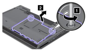
5. Remove the screws that secure the keyboard.
