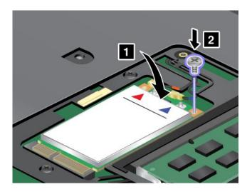
10. Connect the antenna cables to the new PCI Express Mini Card as shown in the drawing.
