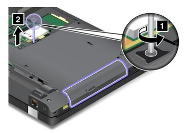
6. Press the edge of the optical drive outwards, using the tip of a thin screwdriver as shown in the drawing and then pull out the optical drive.
