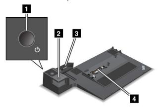
1 Power button: Press this button to turn the computer on or off.
