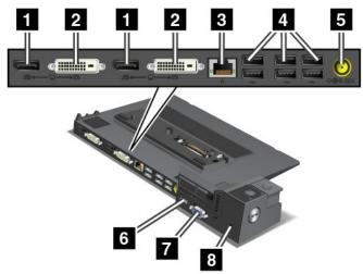
1 DisplayPort connector: Connect a display device.
