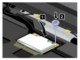
10. Connect the cables to the new wireless LAN/WiMAX card. Be sure to attach the gray cable to the connector marked **TR1** or **Main** on the card, and the black cable to the connector marked **TR2** or **Aux**.
