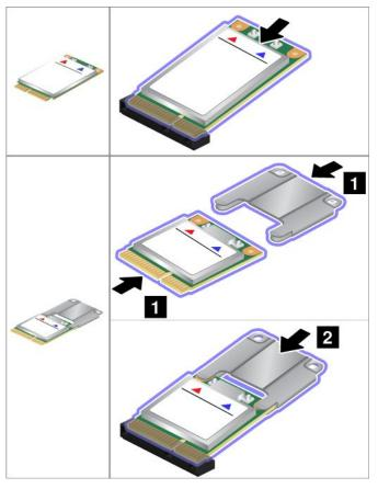
9. Pivot the card until you snap it into place. Secure the card with the screw.
