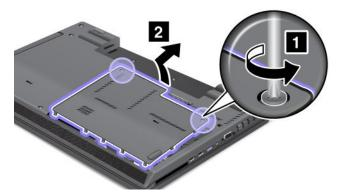
5. Loosen the screw that secures the optical drive and remove it.
