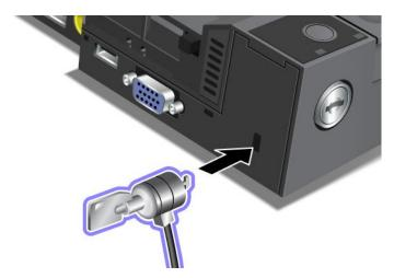
Attach a mechanical lock to the ThinkPad Mini Dock Series 3 or Mini Dock Series 3 with USB 3.0 as shown:
