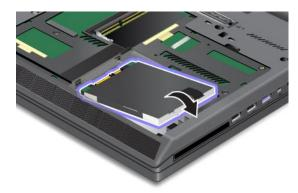
8. Slide the hard disk drive or solid-state drive firmly into place.
