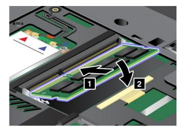
Note: Insert the memory module into the socket at an angle of about 20 degrees.
