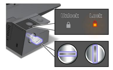
When the key is in the locked position, the eject button of the ThinkPad Mini Dock Series 3, ThinkPad Mini Dock Plus Series 3, Mini Dock Series 3 with USB 3.0 or Mini Dock Plus Series 3 with USB 3.0 is locked, and you cannot remove your computer. The key lock indicator lights when the eject button is locked.
