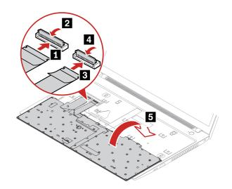
2. Insert the keyboard into the keyboard bezel as shown. Ensure that the top edge of the keyboard (the edge that is close to the display) is under the keyboard bezel.
