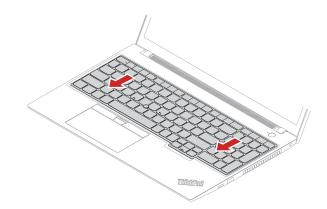
4. Tighten the screws to secure the keyboard. For L14 Gen 3
