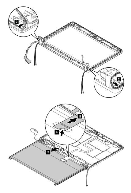
When installing: Make sure that the LCD connector is attached firmly.
