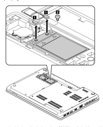
When installing: Plug the red cable into the jack marked MAIN, and the blue cable into the jack marked AUX on the card.
