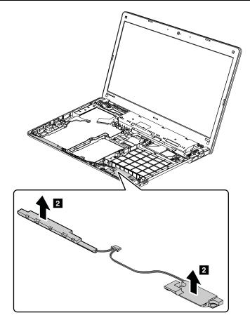
When installing: Attach the speaker assembly and route the cable as shown in the following figure, and make sure that the speaker connector is attached firmly.
