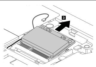
When installing: Plug the gray cable into the jack marked MAIN or M, and the black cable into the jack marked AUX or A on the card.
