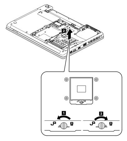
When installing: Place the CPU above the CPU socket, and then rotate the head of the screw in the direction shown by the arrow 3 to secure the CPU.
