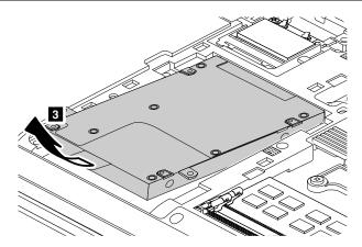
When installing: Make sure that the hard disk drive is attached firmly.
