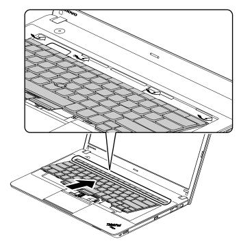
3. To make sure that the front side of the keyboard is housed firmly, gently press the keys with your thumbs and slide the keyboard toward you until the keyboard is in place.
