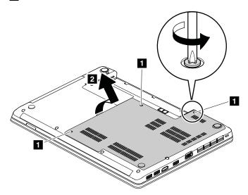
When installing: Attach the large bottom cover as shown in the following illustration.
