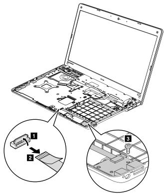
When installing: Make sure that the connector is attached firmly to the system board.
