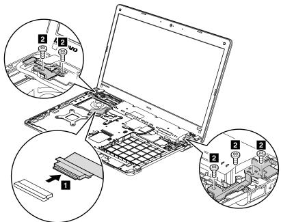
When installing: Make sure that the connector is attached firmly to the system board.
