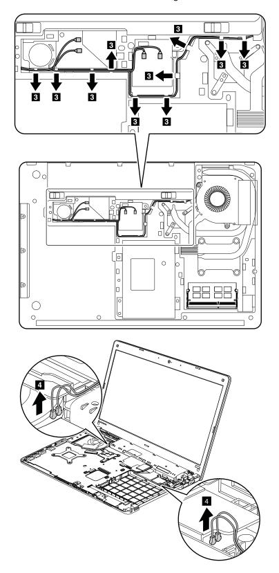
In step 5, release wireless antenna cables from the cable guides.
