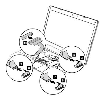
When installing: Make sure that the connectors are attached firmly to the system board.
