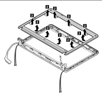
When installing: Make sure that all the latches are attached firmly. Then secure the bezel with the screws.
