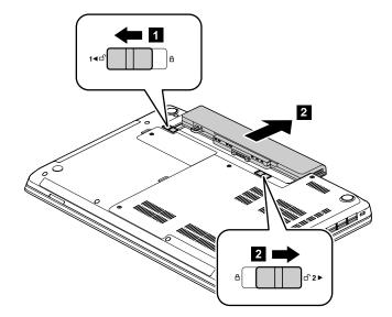
When installing: Install the battery pack in the slot. Make sure that the battery latch is in the locked position.
