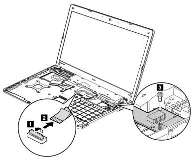
When installing: Make sure that the connector is attached firmly to the system board.
