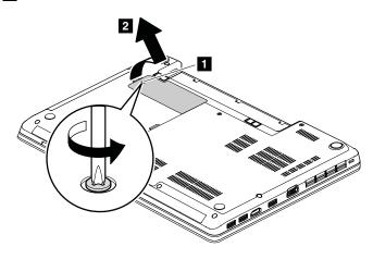
When installing: Attach the small bottom cover as shown in the following illustration.
