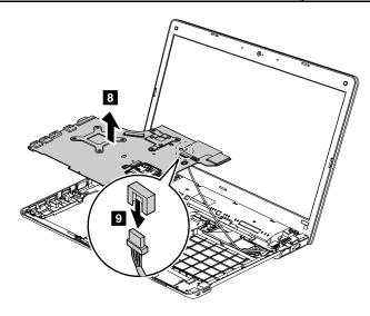
When installing: Make sure that the connector is attached firmly to the system board.
