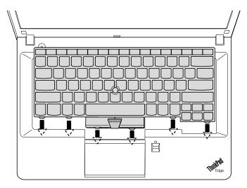
4. Secure the keyboard by tightening the screws from the bottom side of the computer.
