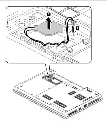
When installing: Make sure that the connector is attached firmly.
