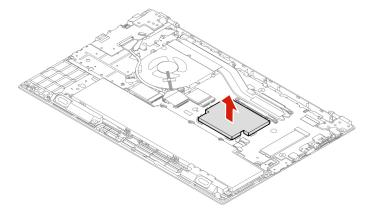
6. Open the latches on both sides of the memory module slot at the same time **I**, and then remove the memory module 2.
