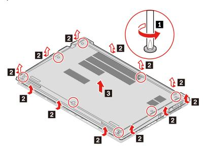
5. Install the new base cover assembly in place 1. Ensure that the latches of the base cover assembly are secured under the base cover assembly 2. Then, tighten the screws to secure the base cover assembly
