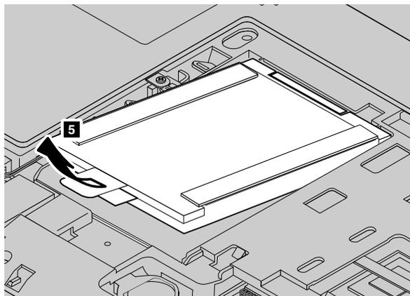
7. Slide a new hard disk drive firmly into place, and then reinstall the screw to secure the drive.
