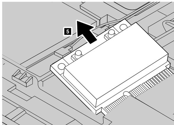
7. Align the contact edge of the new PCI Express Mini Card with the corresponding socket.
