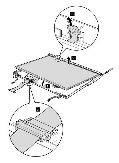
**When installing:** Make sure that the LCD cable and the cable guide are attached firmly as shown in **a**.
