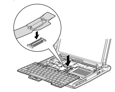
2. Attach the keyboard so that the keyboard edges **a** are under the frame as shown in this figure.
