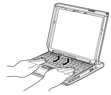
4. Secure the keyboard by tightening the screws from the bottom side of the computer.
