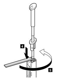
In step **5**, detach the rod antenna from the antenna cable.
