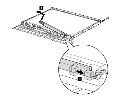
When installing: Make sure that connectors **2** and **3** are attached firmly.
