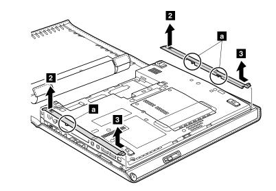
When installing: Make sure that the latches on the bottom side of each bezel are attached firmly.
