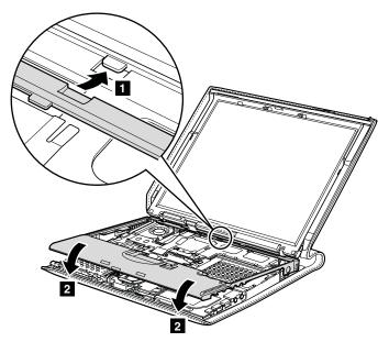
When installing: Make sure that the claw is attached firmly **1**. Then attach the front edge of the keyboard bezel **2**.
