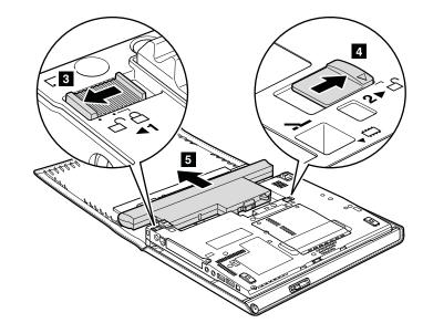
**When installing:** Install the battery pack along the slide rails of the slot. Then make sure that the battery release lever is in the locked position.
