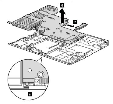
In step **7**, detach the HDD sub card from the system board.
