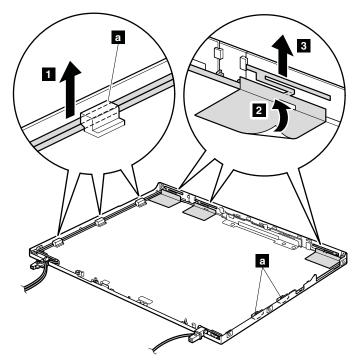
When installing: Route the antenna cables as shown in this figure. As you route the cables, make sure that they are not subjected to any tension. Tension could cause the cables to be damaged by the cable guides, or a wire to be broken.
