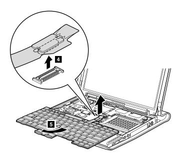
When installing: do as follows:1. Attach the keyboard connector.
