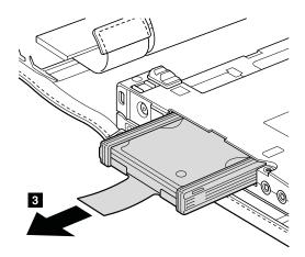
When installing: Make sure that the hard disk drive connector is attached firmly.
