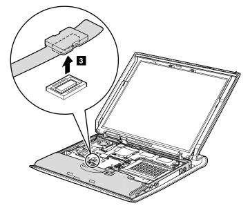
In models with a fingerprint reader, detach the fingerprint reader connector.
