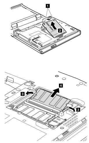
When installing: Insert the notched end of the DIMM into the socket. Press the DIMM firmly, and pivot it until it snaps into the place. Make sure that it is firmly fixed in the slot and does not move easily.
