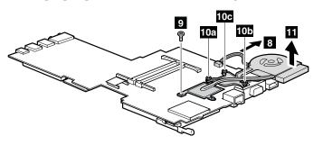
Note: Remove the fansink screws in the order shown 10a , 10b , and 10c .
