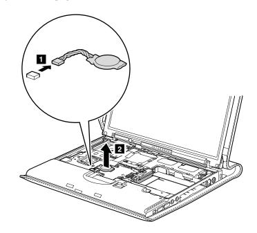
When installing: Make sure that the battery connector is attached firmly.
