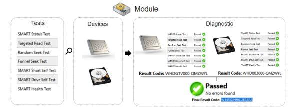
When a diagnostic is finished, Lenovo Diagnostics displays the results for each performed test and create two results codes resuming the test execution.
