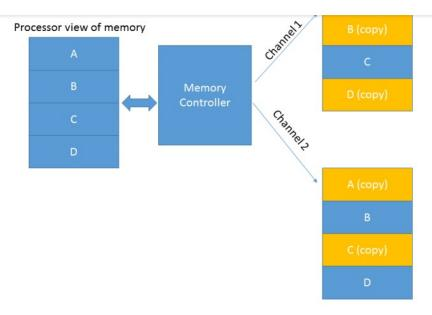
Figure 1: Mirror channel interleave
